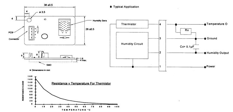
Rx and Cx are both external components, Cx provides smoothing on the humidity output. Temperature measurement can be acheived either by using the resistance of the thermistor and measuring between pins 1 and 4 (see below for formulae) or by connecting a resistor 'Rx' as shown, thereby obtaining a voltage output. ie if  $Rx=50K\Omega$  then at 25°C the voltage on pin 4 would be 1/2 of the supply; 2.5V.
